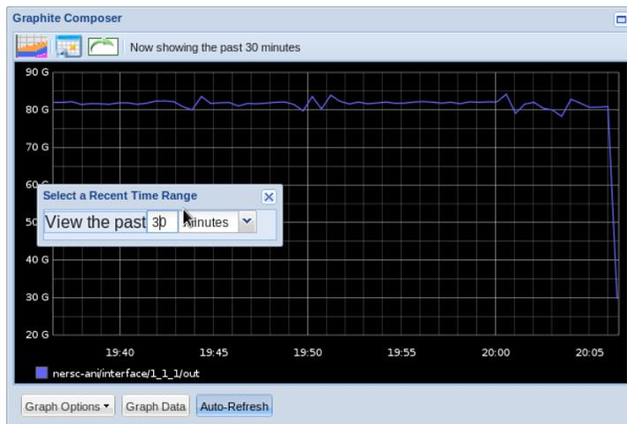
Figure 4: SC11 Climate100 demonstration results, showing the data transfer throughput
